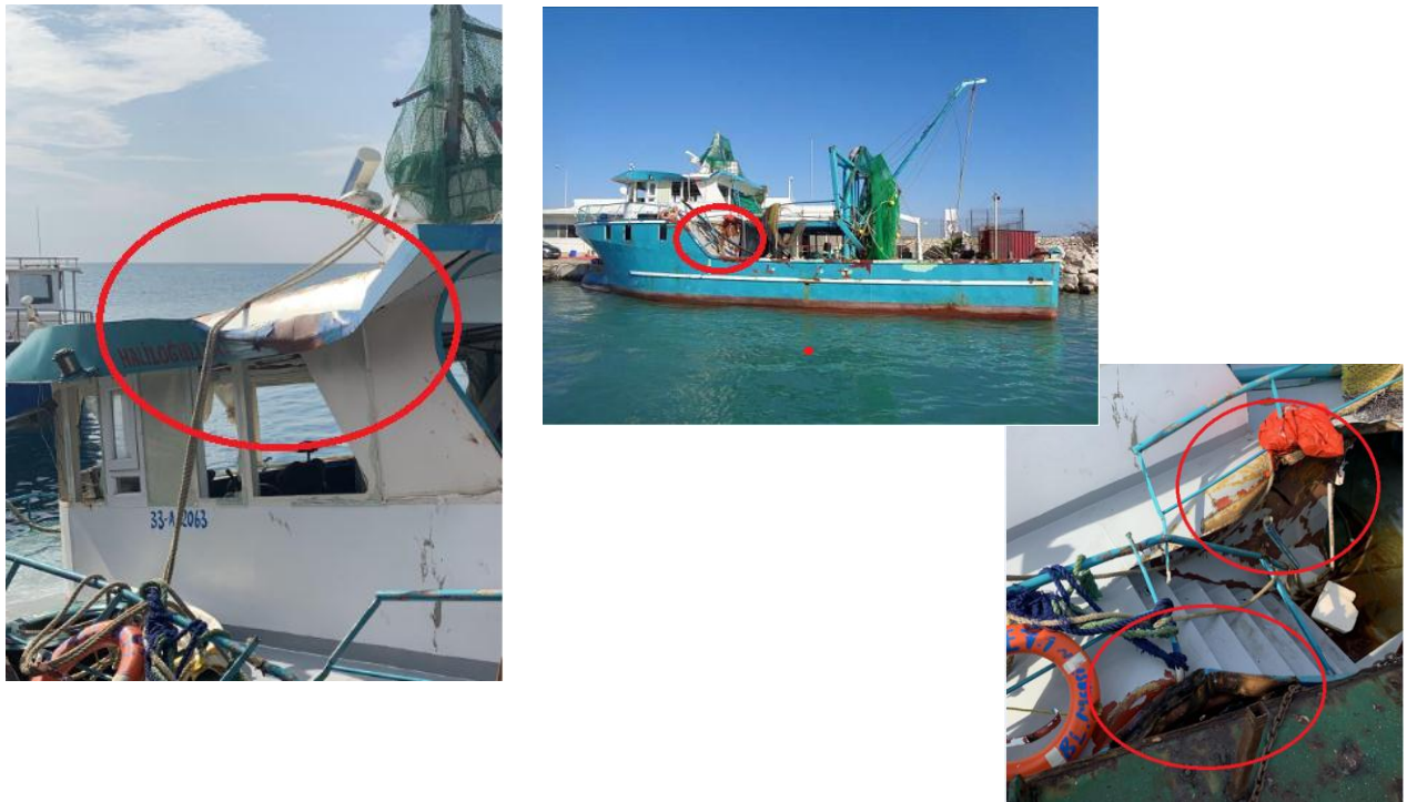
Figure 62: Picture at the right: The damage sustained in the wheelhouse superstructure of POLAT BEY 1. Pictures at the left: Damaged area of POLAT BEY 1
