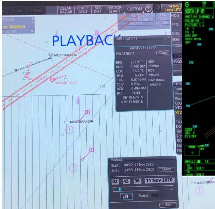
Figure 38: ECDIS data at 05:42:36 Figure 39: APRA recording at 05:42 CPA:0.071 nm; TCPA:03:25 min; BCR: -0.484 nm
